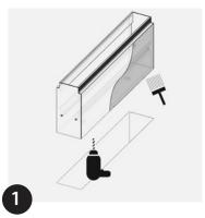
Drill for power cable entry (10mm/ 0.39" min). Coat aluminium box against corrosion if required. Install KKFR-03 ground box in floor slot and level to finished floor surface.
